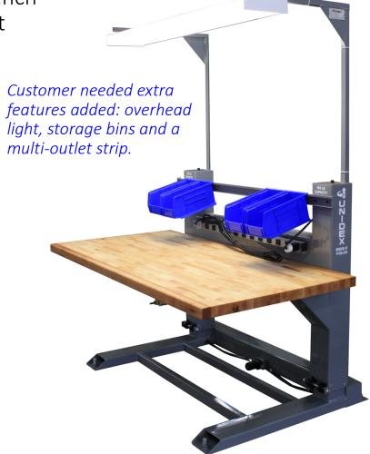
Unidex EHW Series Electric Hydraulic Workbench features an electric hydraulic lift system for instant adjustment of working heights using a foot pedal, toggle switch or pendant.
