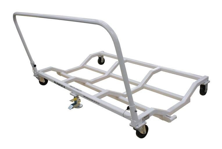
A customer came to Unidex with a unique problem. They needed help putting the cardboard sleeves on the long heavy shafts before storing on the rack. This device has straps to secure the sleeve and using an onboard winch, it pulls the shaft through the sleeve. Slots on the cradle allowed for access to lift the protected shaft.
