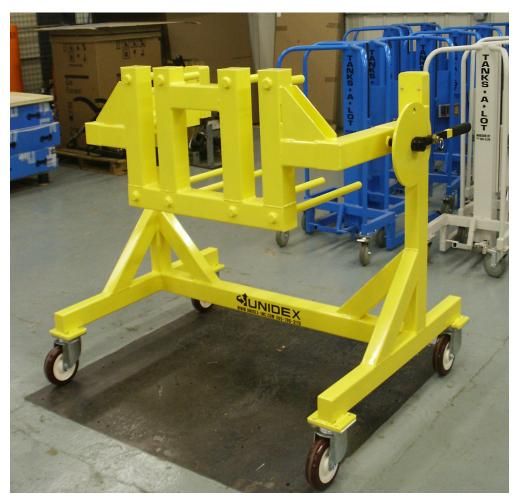
This cart that supports up to two rolls, supported by the core. The rolls are moved directly to the machine at the spindle height where they are manually pushed off. The cart weight capacity is 400 lbs, able to support two rolls 200 lbs each.
