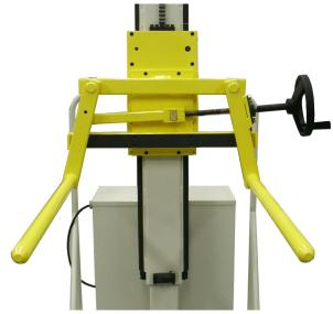
Another feature we can add to a simple probe is a small wheel at the end that offers a wheel to give the operator some leverage when manually loading or unloading the roll. The task of moving the roll is much easier with this feature.
