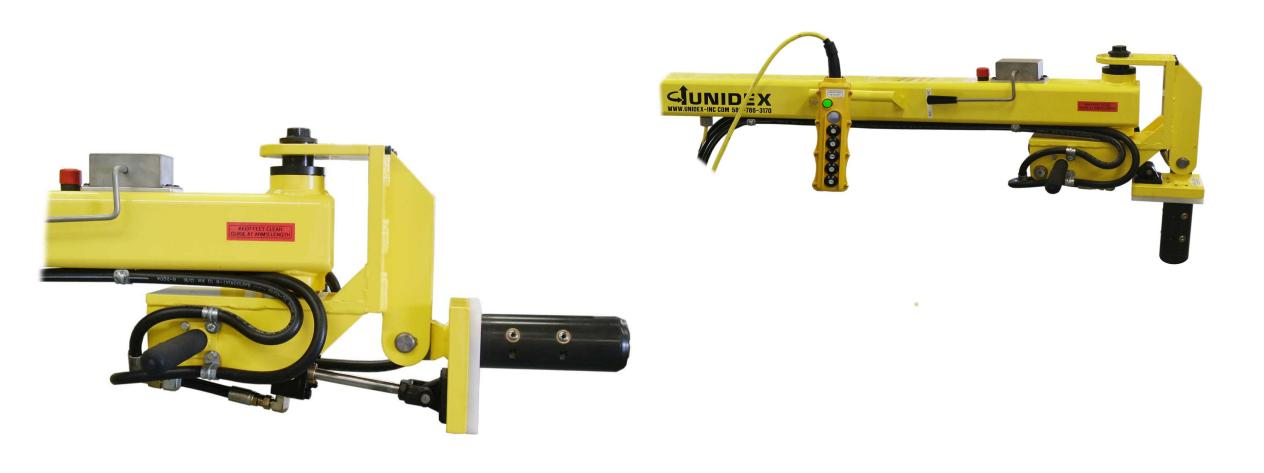
Sometimes rolls are not heavy but they are a sensitive material. This is a lightweight core gripper and the operators are not able to touch the roll material. The rolls were 20 lbs. and this is mounted on a light duty manipulator with an articulating arm.
