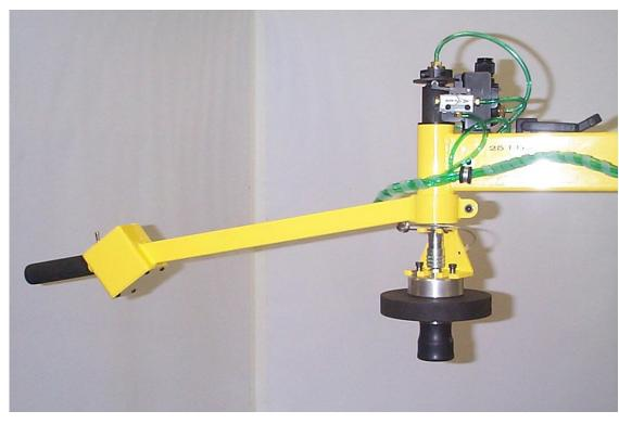
Shown is two manually adjusted support arms that pick a variety of sizes of rolls from the bottom. This application is designed for textile rolls that do not have a core. A hand wheel operated a left and right hand screw that allows the arms to adjust to the roll sizes. It is shown on our PE Model.
