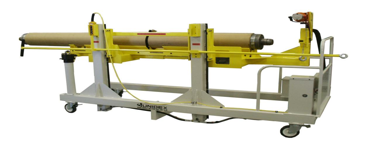
This end tool supports a roll by the core and has an air powered pusher plate for unloading. The roll weight is 300 lbs and this tooling attaches to our PE Model Lift that has a power lift and manual push.
