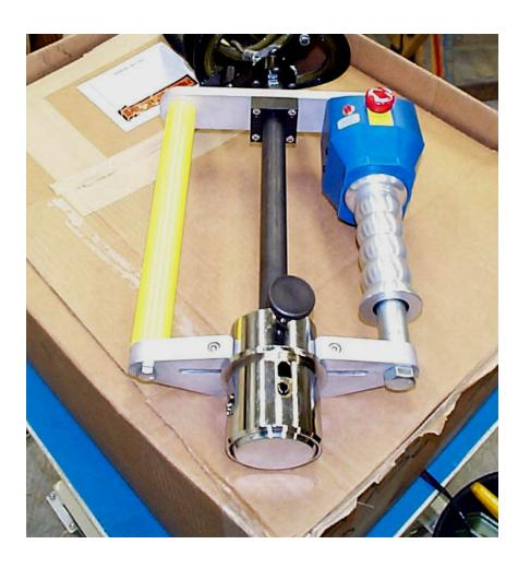
This powered core gripper that we developed is mounted on our ECL Manipulator. It offers a power grip and a power upend. Typically it is used to pick rolls with the core horizontal, lift and rotate down to put on a pallet. This gripper can easily handle rolls up to 350 lbs.
