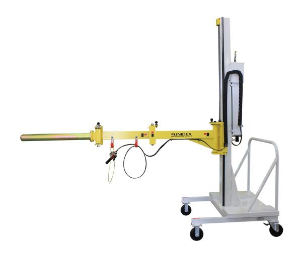
This cart supports 2 rolls getting loaded from a storage rack by a hoist with a core gripper. They are transported to the machine where the operator manually rotates the rolls 90 degrees (using the black lever) to offload on the spindle. The rotator was designed on the centerline of the rolls to allow an easy rollover with a max 500 lb capacity.
