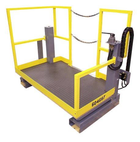
This single-person lift is positioned in front of a sand blast cabinet for the different height operators to easily see inside while blasting.
