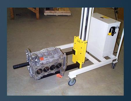
PE Series workstations are designed for your specifications; whether you need gripper action, a boom arm with 180° of swing or sliding forks.
