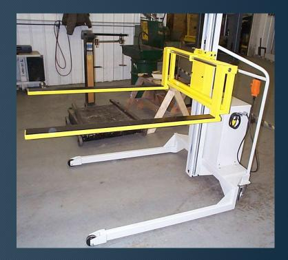
PE Series workstations are designed for your specifications; whether you need a cradle, a boom arm with 180° of swing and indexing or forks for lifting delicate items.
