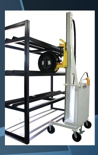
A manual rotation with positive locking positions, approximately 12 positions in a 360° rotation. End tooling has 4 pins attached to a bolt plate with a Destaco-type clamp that secures part.
