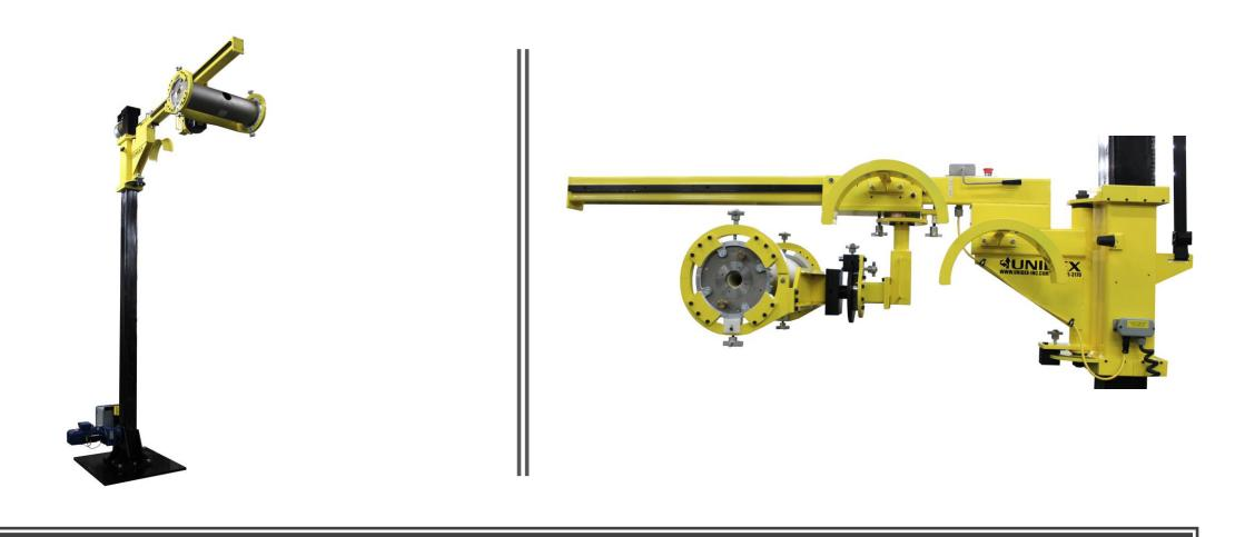
Shown above is a highly custom end tool to support an XRAY machine for checking welds. The end tool allows the Xray machine to be positioned and locked in place as the part is moved to check the welds. Included are holders to support the wires and cables.
