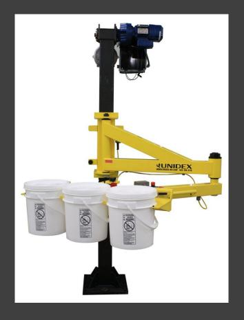
One of our customers added a new filling line and asked for help to pick and place full buckets of peanut butter to stack on pallets. These filled containers are heavy and bulky to handle during an 8-hour shift.
