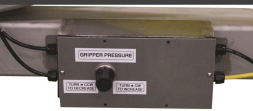
Here is a Stainless Steel ECL Manipulator with a powered gripper designed to pick fiber drums. Included on the gripper was controls to increase or decrease the grip pressure on the drums. This Manipulator is in the Food Industry where it is frequently cleaned and wiped down. The weight capacity is 650 lbs. at the end of the arm.
