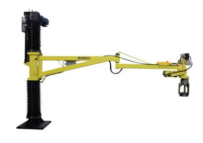
This is an ECL Manipulator designed to assist operators to replace dies in a machine at a steel mill. Due to the environment, bellows were added to the column to protect the moving parts on the lift mast. The three-jaw gripper contacts the dies on the groove.
