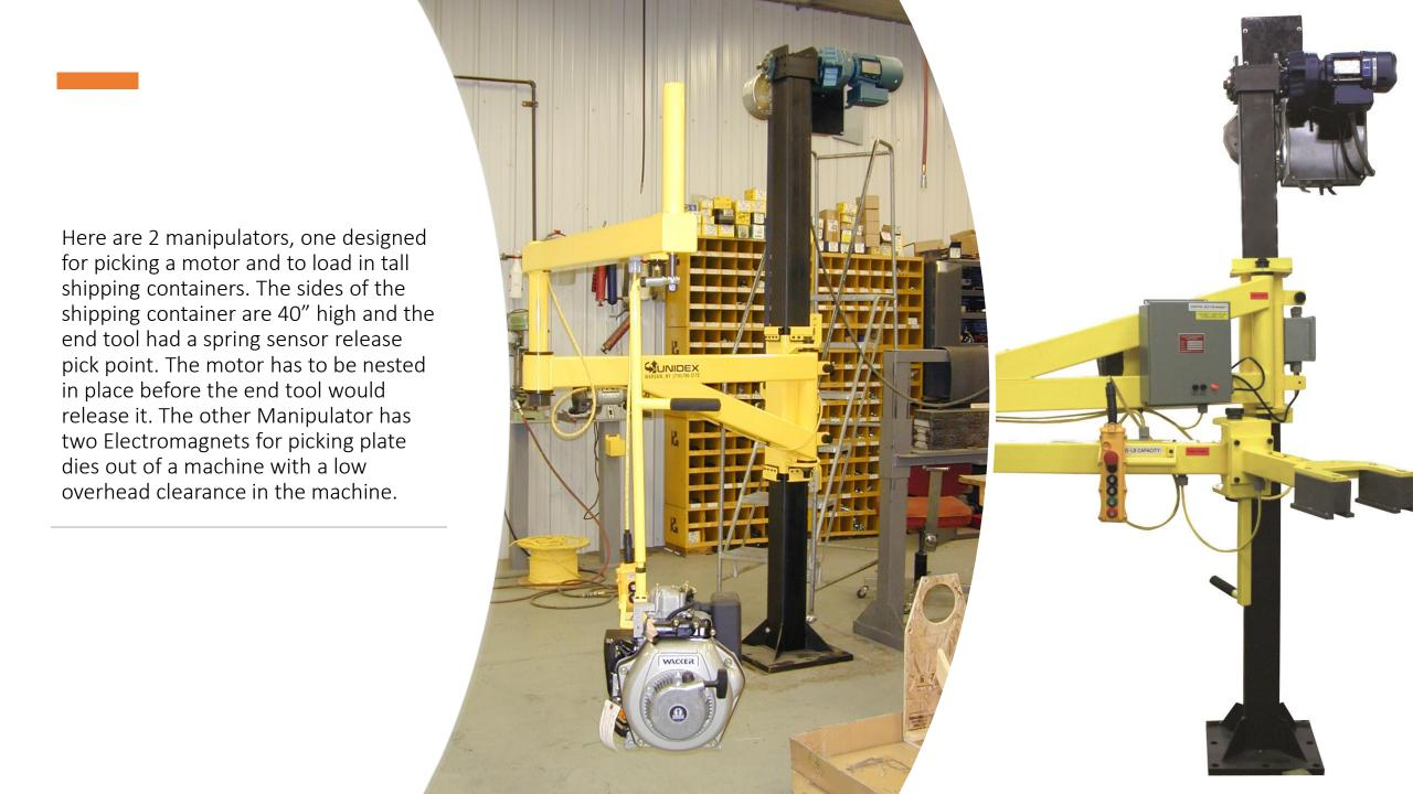
On occasion, customers need a Manipulator on a portable base. The base requires a fair amount of counterweight relative to the load capacity and arm length. Ideally it is best if the load is less than 100 lbs. and the reach is less than 8'. The gear motor is mounted at the bottom to act as counterweight.
