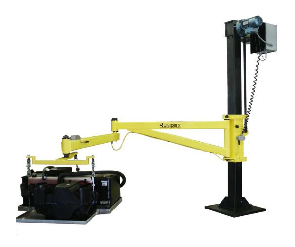
Here is a manipulator we designed to pick and hold a fan blade. The fan blades come into the assembly area on a cart standing upright and need to be picked, rotated and manipulated for install. These fan blades are approximately 50 lbs each. The end tool has a vacuum cup with two axis of rotation to position as needed.
