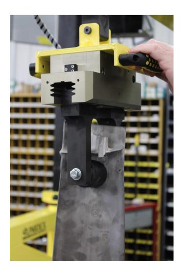
Here is a manipulator mounted to a riser so the operator can stand behind the end tool and control rotation and positioning of the gripper. The application involved picking various shapes of sand castings off a conveyor and placing them into a machine.
