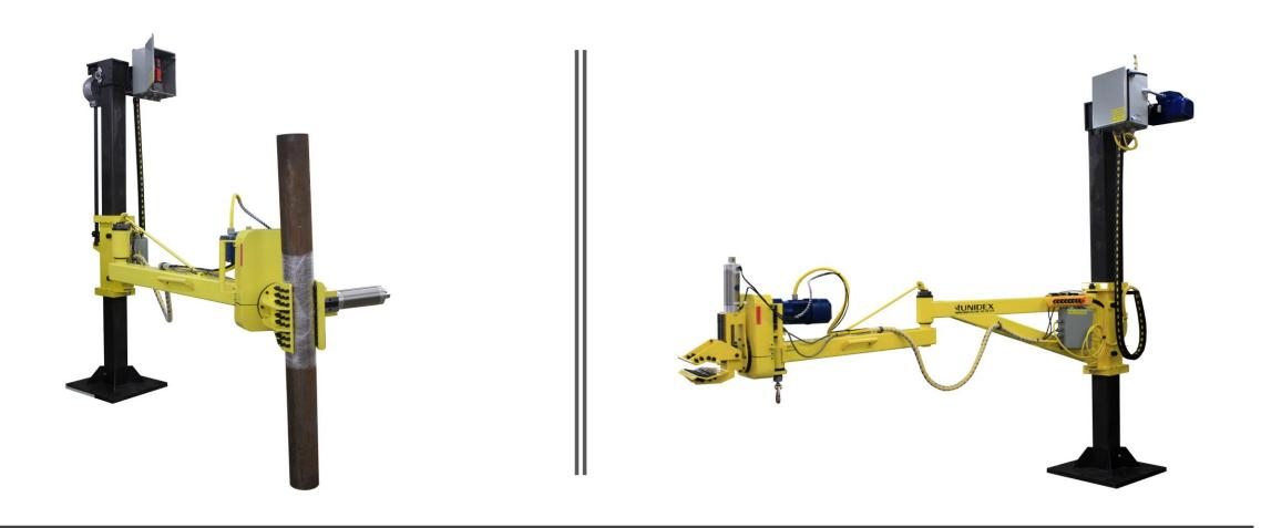
This ECL Manipulator was designed to pick a cylinder out of a bench type cradle and rotate it 90 degrees to insert into a vertical tube. The picture shows a steel tube to simulate the cylinder. The cylinders weigh up to 300 lbs each we designed an air-powered grip with an electric gear motor for the rotation. The arm provides 8' of reach.
