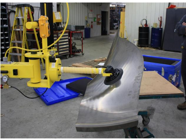
One of the big challenges is providing an end tool that will work for each customer's problem. The manipulator you see below picked a fan blade but needed to only be picked and placed. The gripper we chose has rubber contact pads to prevent any damage to the part but offers a strong grip.
