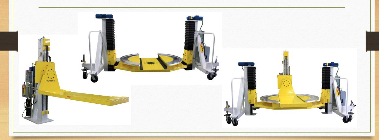
EH Positioner that secures and rotates a 4000-lb. engine for assembly, from a horizontal position to vertical.
