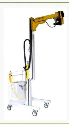
A variety of carts allow for proper height adjustments. (L) Manual Push Cart with manual tilt and rollers to support large rings. (M) Portable Lift to support large ring for fan case housing. (R) Powered Trunion Cart towed with a fork truck.
