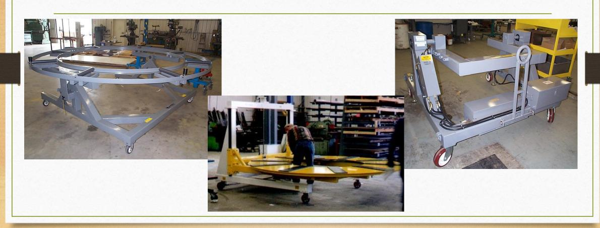
Floor mounted Electric Hydraulic Lift with rotation that interfaces with a cart to lift a composite fan case.
